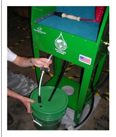
**Step 10**: Pour 5 Gallons of distilled water (or approved paint company waterborne gun cleaning solution) slowly into the sink with one well shaken bottle of BECCA Water Wave additive.
