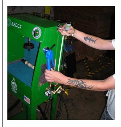
**Step 8**: Install a fitting into the ball valve on the air regulator that is compatible with the shop air (due to a variety of applications, this part is not supplied by BECCA).
